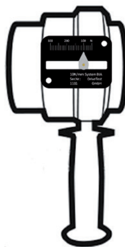
Analysis via mechanical trailing pointer concurrent with measurement
